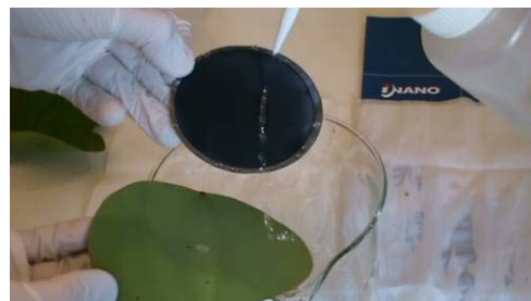
Figure d9. A still from the NANOYOU Video 4-Lotus Effect ® -Part 2 where a piece of porous silicon is compared to a real Lotus leaf. (Image credit: L. Filippini, iNANO, Aarhus University, Creative Commons Attribution ShareAlike 3.0)
